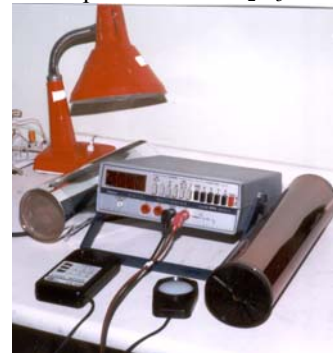
Fig. 8. Photoreceptor resistance measurement upon exposure to light.
