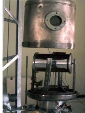
Fig. 6. Al deposition and \text{Al}_2\text{O}_3 formation.
