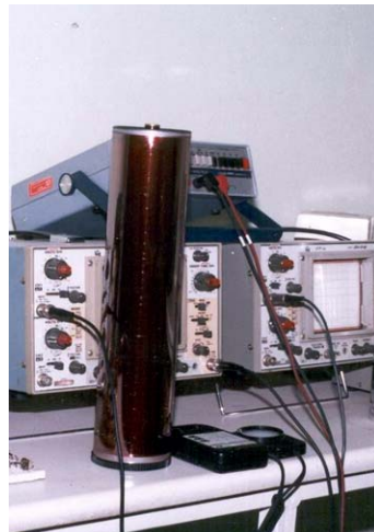
Fig. 9. Photoreceptor resistance measurement in dark.
