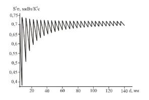
Figure 1. Theoretical dependence of the thermoelectric power  $S^2\sigma$  from the thickness d of thin films of n-PbTe at T = 300K
